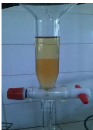
a. Settling of Hura crepitans ' biodiesel after washing
